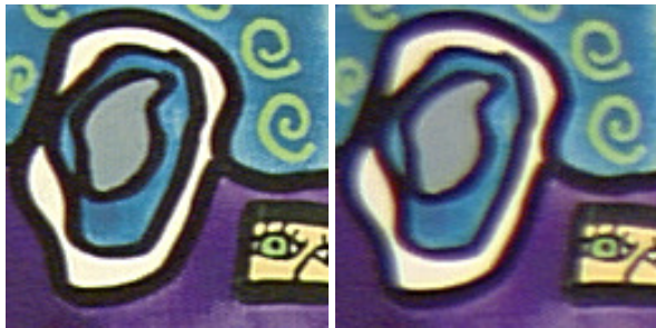
Figure 8. Part of the test image pair B^{50\%} . The autoiris -function of the camera compensates the illumination intensity change from 100% to 50%
