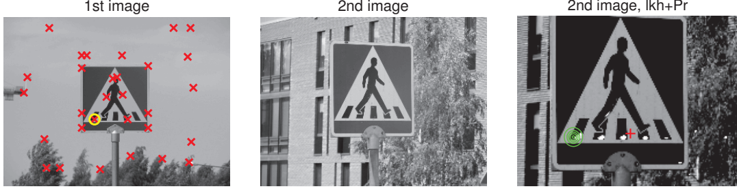
Figure 2. Left image: starting image and its node set. Middle image: second image in the sequence. Right image: zoomed second image, with white fields showing the modes of the likelihood of a node, marked with yellow circle in the starting image, and green contours illustrating the marginal prior distribution of the node (given scale 1.32, orientation -0.10^\circ , and the midpoint, shown as red cross).
