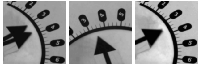
Figure 6. Subframe warping synchronization. Left: two consecutive overlaid fields from first camera. Center: closest integer frame aligned field from second camera. Right: warped field from first camera, synchronized to match the second.
