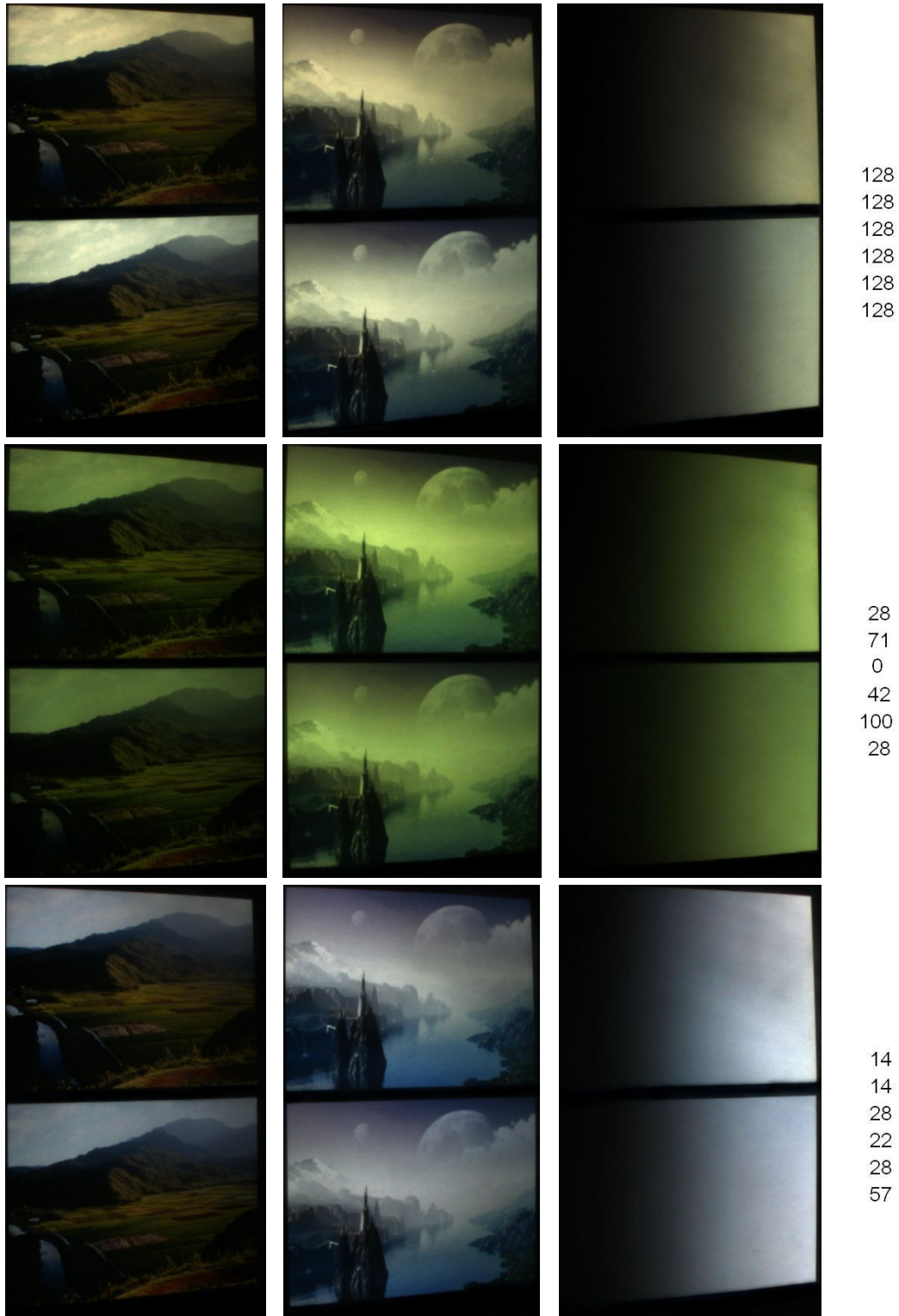
Figure 3. Comparison of displayed results for several hardware adjustment settings. Each of the three rows shows the results for a pair of projectors stacked on top of each other. Three different images are shown in each row for comparison. The older projector illuminates the upper half of each image; the newer projector displays the lower half. The far right column shows the 3-channel contrast settings for each of the two projectors. (Top Row) Images are shown with the default hardware settings. (Middle Row) Hardware settings for optimum of cost function with W_m = 1 , and all other weights zero. Notice that the projectors match each other better than with the default settings, but the results appear yellowish. (Bottom Row) Hardware settings for optimum of cost function with W_m = 1 , W_b = 1 , W_g = 0 , and W_i = 0 . The projectors match each other well and a white balance close to the desired one is achieved.
