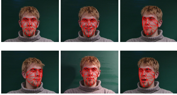
Figure 2. Sample images for a subject in the IMM Face Database with the mesh connecting facial landmarks superimposed.
