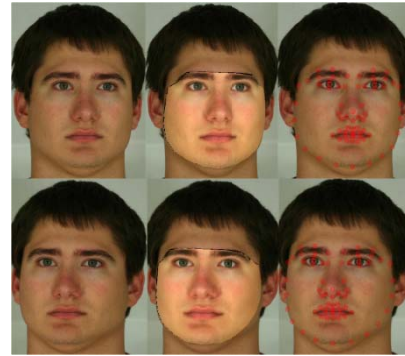
Figure 5: AAM fitting results for a probe at 3 meters. First column is the input image. Second column is the final AAM result with superimposed best-fit texture. Third column shows final AAM vertices.
