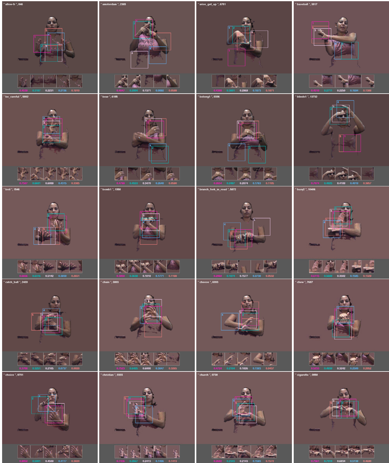
Figure 6. We show hand detection results using the 13 neighborhood aligned distance based detector on gestures with interacting hands from the LAB-F set. The training and test setup for this experiment is described in Section 7.3. The detection scores (i.e., SVM outputs) for top five hand ROIs are displayed for each frame sorted in decreasing order.
