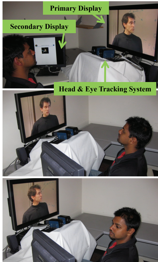
Figure 3. Setup of the Intelligent Room experiment. Note the subject has to maintain focus on the primary monitor while checking the secondary monitor under certain conditions. The head and eye motion is tracked using a commercial eye tracking system.
