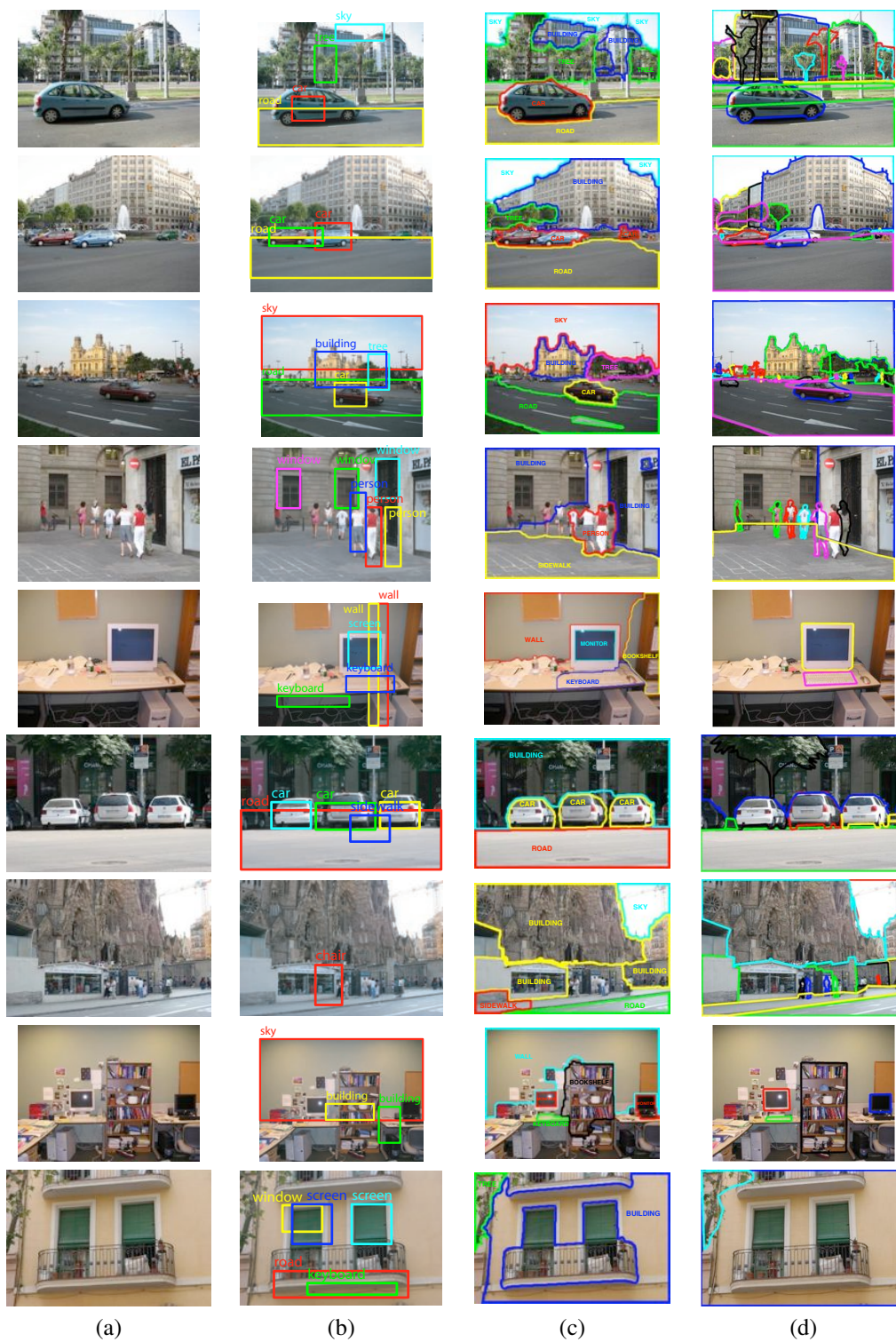
Figure 5. Recognition results for example from LabelMe dataset. (a) Original image. (b) Detected objects by Gist. (c) Recognized objects by CoLA. (d) Ground truth object labeling. Best viewed in color.
