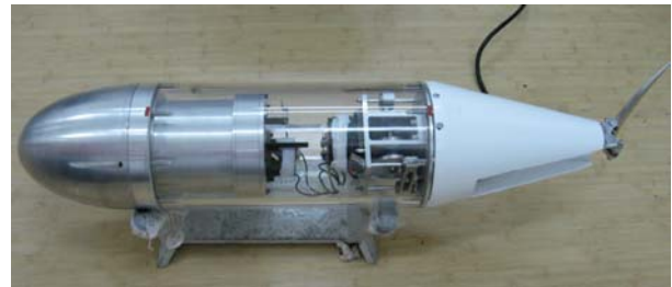
Figure 1. Prototype of rigid robot fish (HRF-II). This prototype appears the body side-sway problem under a test.
