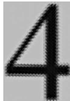
Figure 5. A typical example of reconstructed image with misalignment (with a position measurement error of 0.3 pixels)
