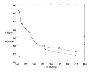
The point "box" in this chart is the point set on Pareto front is given by ST-GA; the point "lap" is the point set on Pareto front is given by Fuzzy-GA; "Triangle" is the ideal point. It is obviously that Fuzzy-GA method is superior to ST-GA in solving Pareto front.
