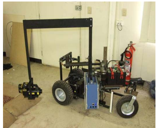
Figure 2(a) X-Ray Inspection Robot
