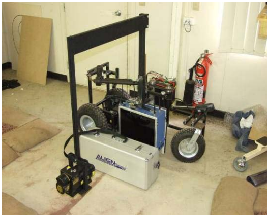
Figure 2 (b) X-ray Inspection Robot in Position to Inspect Luggage
