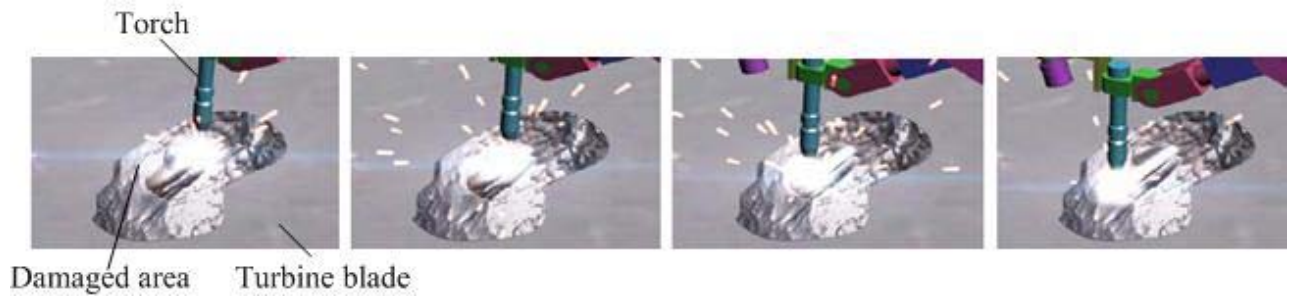
(b) Images of the welding process
