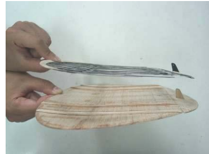
Figure 3 The flexible wing (upper) and the rigid wing (below) with the same shape and the same size. Rigid wing is made by hard wood, strengthened by rib, and with a thickness of 1.5mm.
