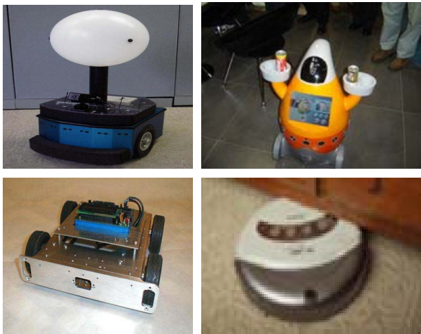
Figure 1. Mobile robots (clockwise from top left): Hearing Robot [5]; Serving Robot [6]; Line Tracking Robot [7]; Roomba Vacuuming Robot [2].
