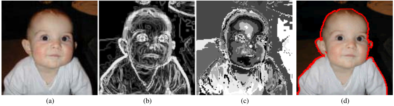
Fig. 4. Segmentation of color homogeneous image. (a) Original image. (b) Edges detected in (a). (c) Primitive regions with region growing method ( \sigma = 8 , 97 regions). (d) Final segmentation ( \sigma_1 = 1 , \sigma_2 = 0.1 ).
