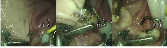
Figure 7. Slave manipulator inside a pig stomach during animal trial
