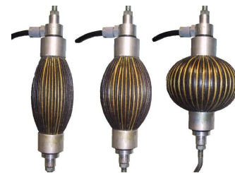
Figure 1. A Pleated Pneumatic Artificial Muscle (PPAM) shown for three different values of contraction.
