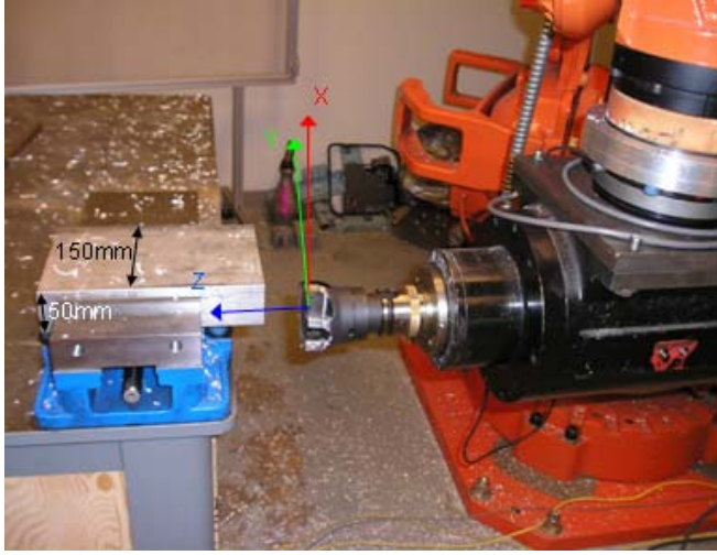
Figure 1. Robotic end milling process
