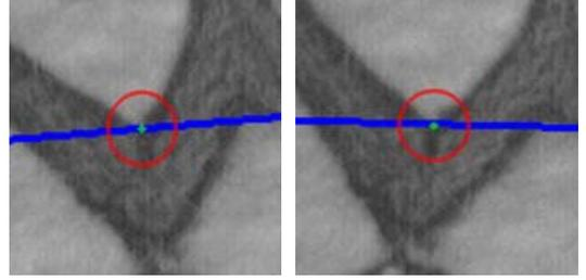
Figure 2. Epipolar lines and neighborhoods (in red circles) illustrations of corresponding points in an image pair
