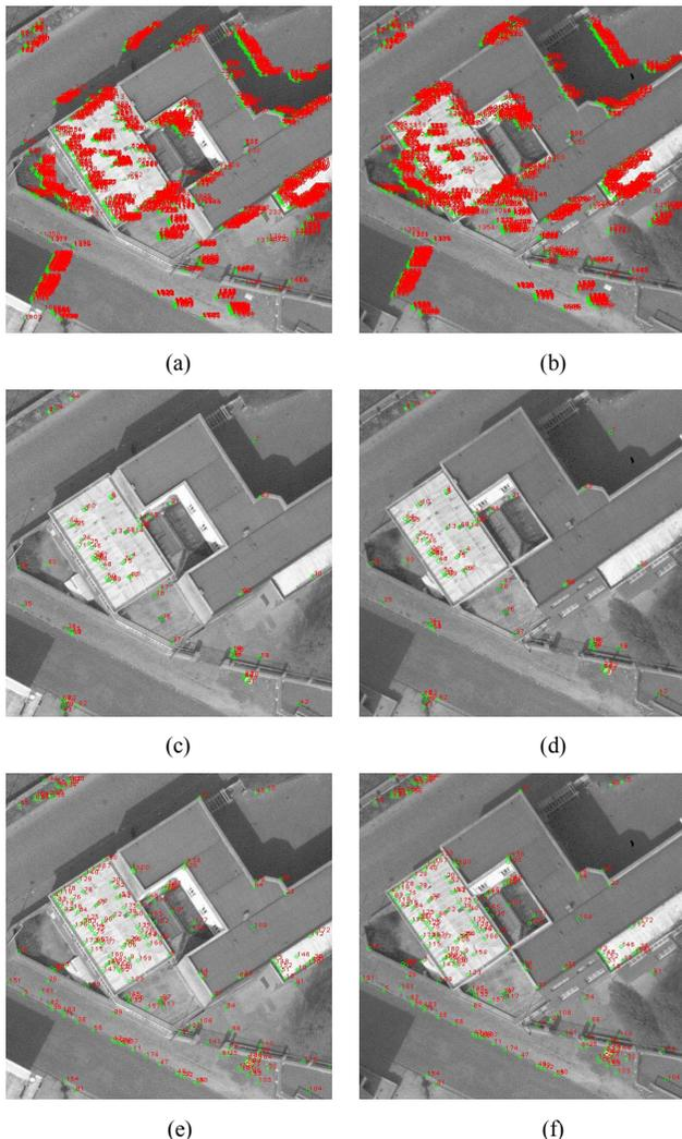
Figure 4. Matches with proposed method (a) and (b), with SIFT (c) and (d), with Harris/Cross-correlation approach (e) and (f), using the aerial image pair
