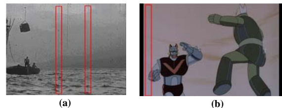
Figure 1. Example of scratches: (a) static/principal/positive scratches (“Sit-down sequence”), (b) a static/principal/negative scratch (“Taekwon V sequence”)
