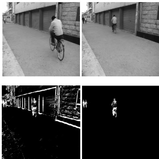
Figure 3. Experimental results of an image from a sequence taken with a shaking camera
