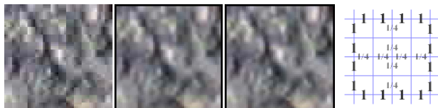
Figure 6. Quantisation blocks: original, 3x3 gaussian blur, quantisation recovery filter, weighting mask
