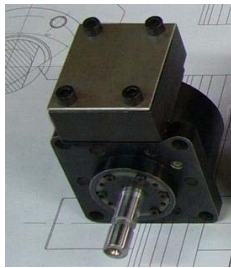
Figure 2. 20Nm loading hydraulic motor
