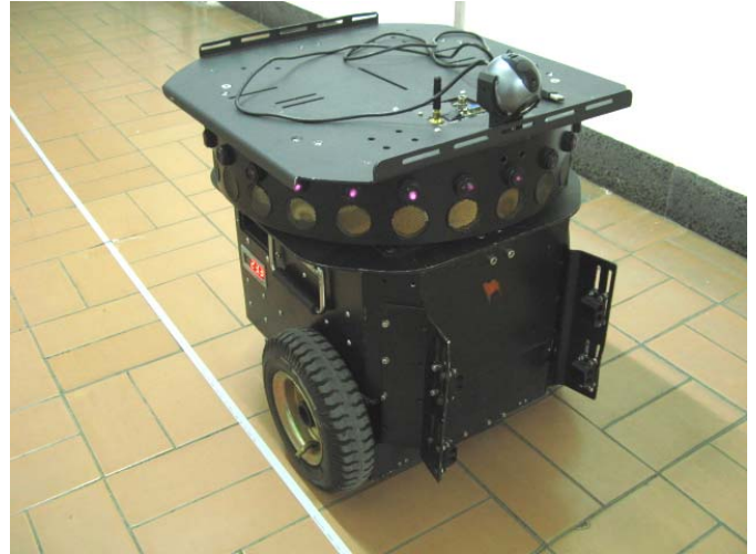
Figure 6. Voyager II type ground wheeled mobile robot
