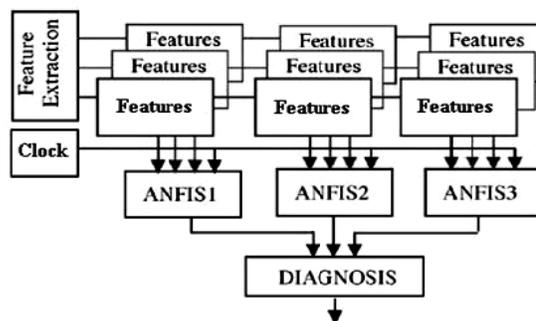
Figure 3. Multiple ANFIS units for multiple fault diagnostics
