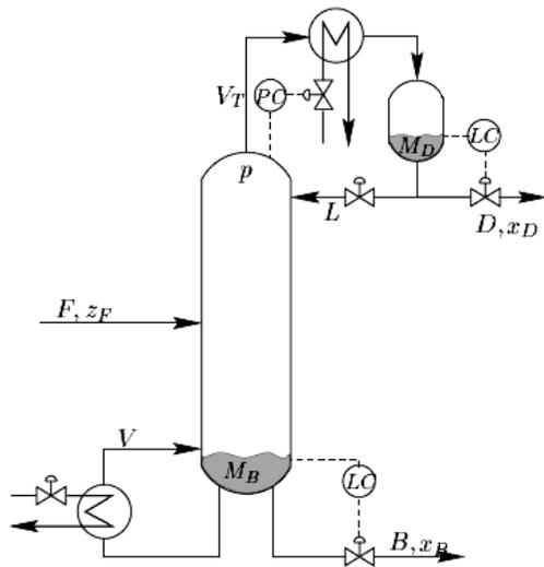
Figure 4. Simple typical distillation column controlled with LV-configuration
