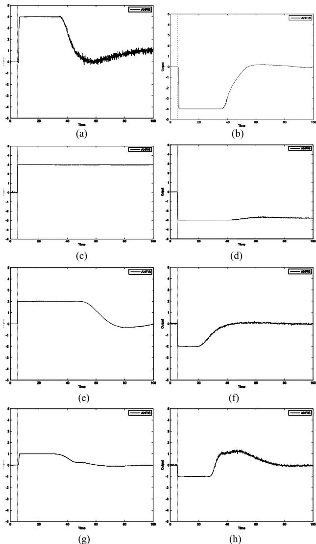
Figure 7. The Fault Diagnosis Function when a fault occurs at feed rate (a),(b) feed composition (c),(d) boil up flow (e),(f) and reflux flow (g),(h) its corresponding fault.
