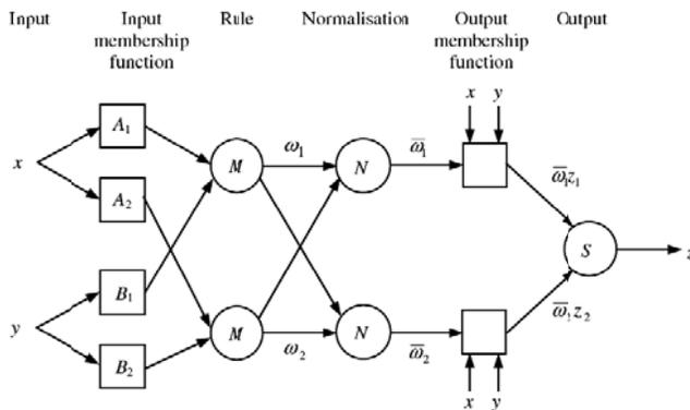
Figure 2. ANFIS structure used in proposed method
