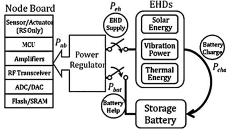
Fig. 1. Power management diagram of a node-board with a battery being supplemented by energy harvesting devices (EHDs).
