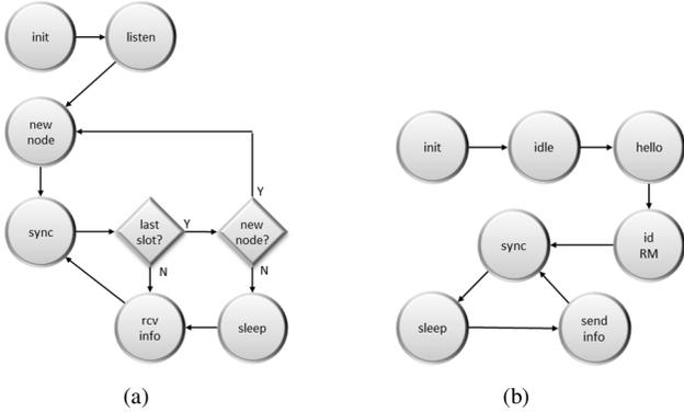
Figure 2. State flowchart of the RAU (a) and SM (b).
