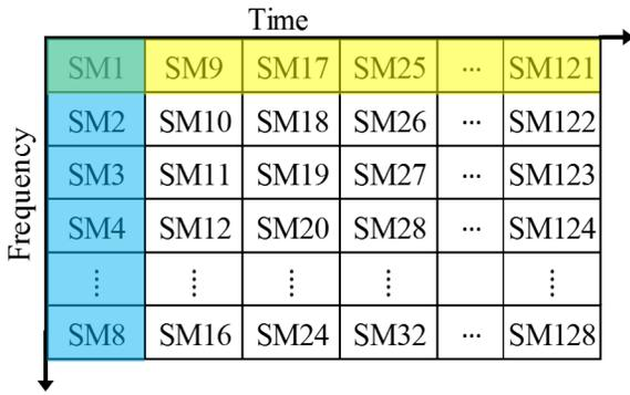
Figure 1. FD-TDMA slot grid.
