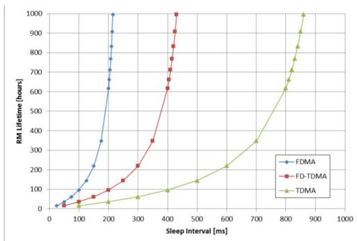
Figure 4. RM Lifetime versus sleep interval.
