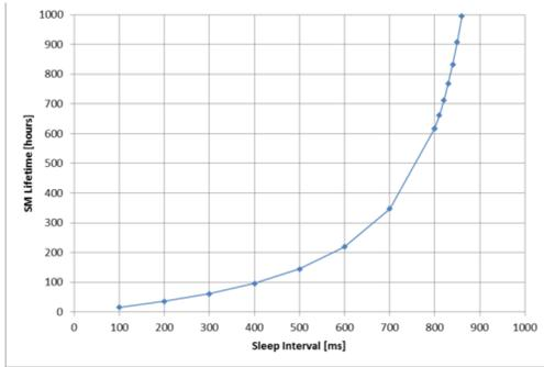
Figure 3. SM Lifetime versus sleep interval.
