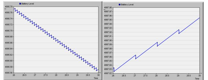
Figure 2. Time samples of the battery level of the SM (left) with  $T_{sleep} = 0.1$  ms and (right)  $T_{sleep} = 1$  ms.
