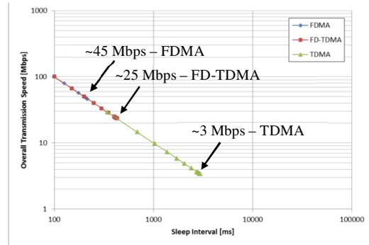
Figure 5. Effective throughput of the multiple access techniques.
