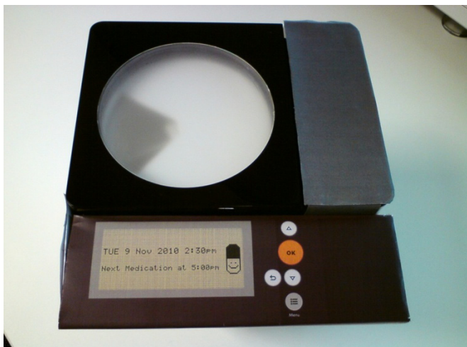
Figure 2. Paper prototype of a human-centered design of medicine dispenser.
