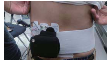
(a) ECG-based HR sensor and its mounting position
