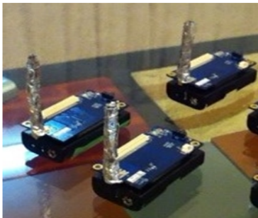
Fig. 2. Modifications to Iris motes to reduce transmission power
