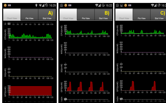
Fig. 7. Intervals of the energy consumption of GPS: uninterruptedly, 30 seconds and 60 seconds, respectively.
