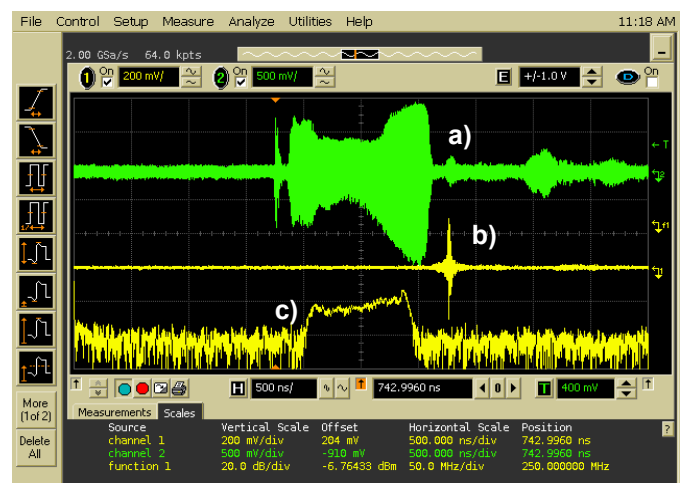
Fig. 1. Time signal of the a) transmitted chirp signal, b) compressed chirp pulse after the matched filter. c) Spectrum of the transmitted chirp signal.
