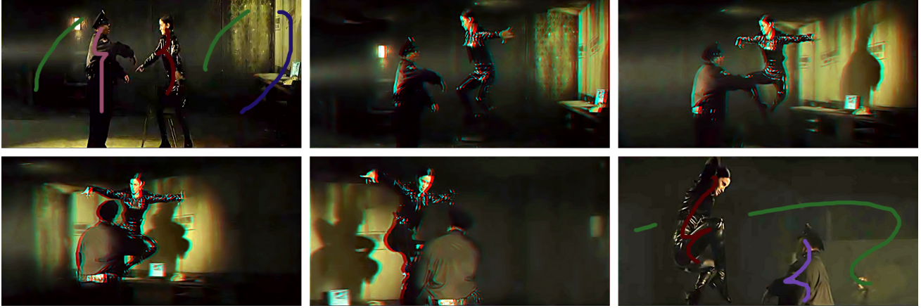
Figure 1. An illustration of the input and output of our conversion system. (from top-left clockwise) original frame from "Matrix" marked by input scribbles; Output, Red/Cyan anaglyph frames form the shot; last frame marked by input scribbles. Note the significant motion of the camera and characters (the full stereo video is provided in the supplementary material).
