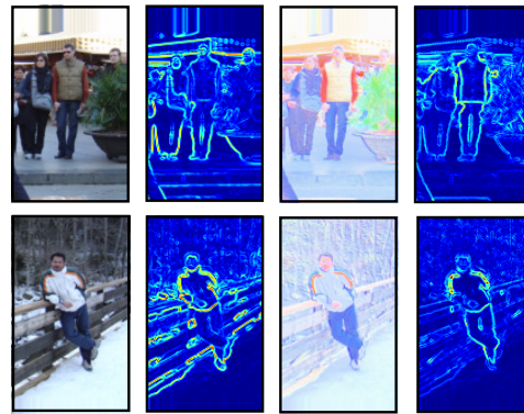
Figure 5. Color normalization. Columns from left to right show: (i) original image; (ii) gradient magnitude of original image; (iii) color normalized image; (iv) gradient magnitude of normalized image. Note how the color normalization is able to suppress background clutter due to intensity invariance and ‘pull out’ the different gradients of the pedestrian.
