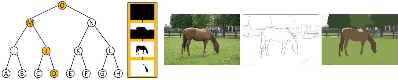
Figure 2. Example of ancestral set. From left to right: • Schematic representation of segmentation tree and example of ancestral set; the leaves are in this case the nodes \{A, B, C, D, E, F, G, H\} and the ancestral set of leaf D is A(D) = \{D, J, M, O\} . • Example of ancestral set on a real image. • Original image. • Hierarchical boundaries produced by the segmentation algorithm. • Finest segmentation, containing the leaves of the tree.
