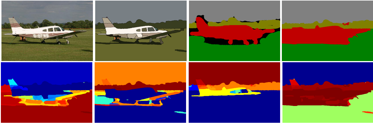
Figure 3. Example of merging the per category confidence maps into a single segmentation. Top: Original image, initial partition, ground truth and final segmentation. Bottom: Confidence maps for the categories grass, tree, sky and aeroplane. The confidence maps of all the categories are used to produce the final segmentation.
