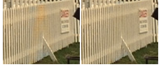
Figure 3. Left: Demosaicking with LSC sometimes causes artefacts such as the yellow and blue pixels in the middle of the fence. Right: The reconstruction obtained with the LSSC algorithm does not exhibit such artefacts. (This figure should be viewed in color.)
