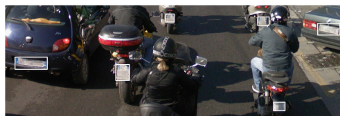
Figure 10. Examples of how ground-truth license plates were marked by humans (in white). Image hand-redacted.
