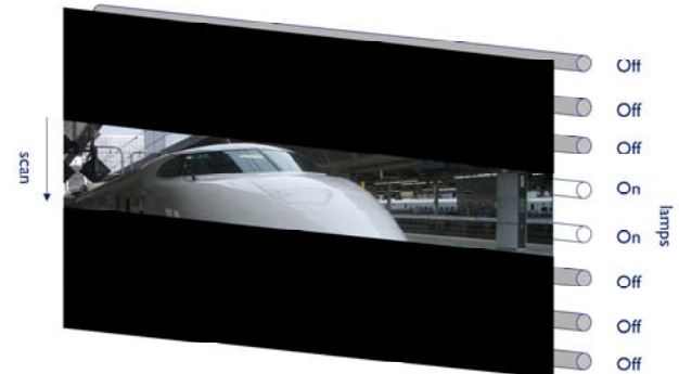
Fig. 2: The scanning mode operation of the backlight. By successive ignition of the lamps a light band scrolls over the screen, once for each frame.
