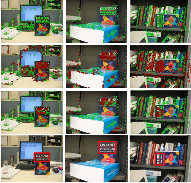
Fig. 2. Pattern discovery result. (1) 1st row: SIFT extraction results, each green point represents a visual primitive p \in \mathcal{D} ( |\mathcal{D}| = 3,084 ). (2) 2nd row: visual primitive pruning results based on individual SIFT matching. Red points are valid visual primitives p \in \mathcal{D}^1 ( |\mathcal{D}^1| = 1,078 ) and green points are those pruned. (3) 3rd row: pattern discovery based on fast spatial neighborhood matching with neighborhood size K = 25 and matching threshold \lambda = 10 . Red points are discovered visual primitives p \in \mathcal{D}^K ( |\mathcal{D}^K| = 316 ) that belong to the common spatial pattern. (4) 4th row: discovered spatial common pattern by fusing the discovered visual primitives.
