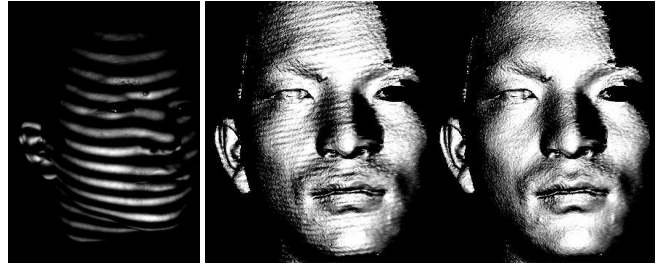
Figure 4: (left) Image of a projected pattern, (center) graphics generated from resulting 3-D models by conventional method, and (right) proposed method.
