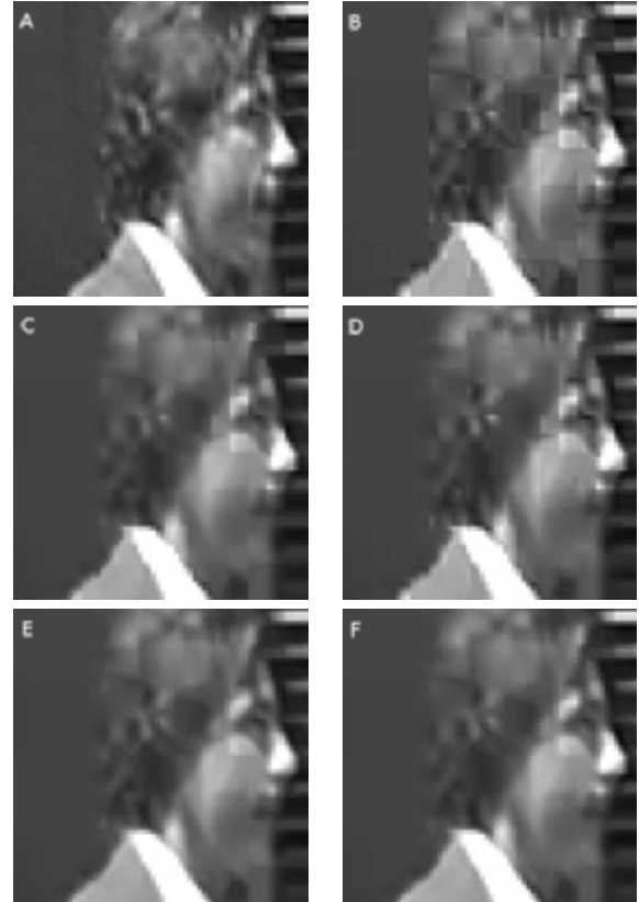
Fig. 6. Image fragments from Hotel sequence: (A) original uncompressed (B) H.264 compressed (C) Bil (D) In-loop filter (E) Pro-l (F) Pro-tb
