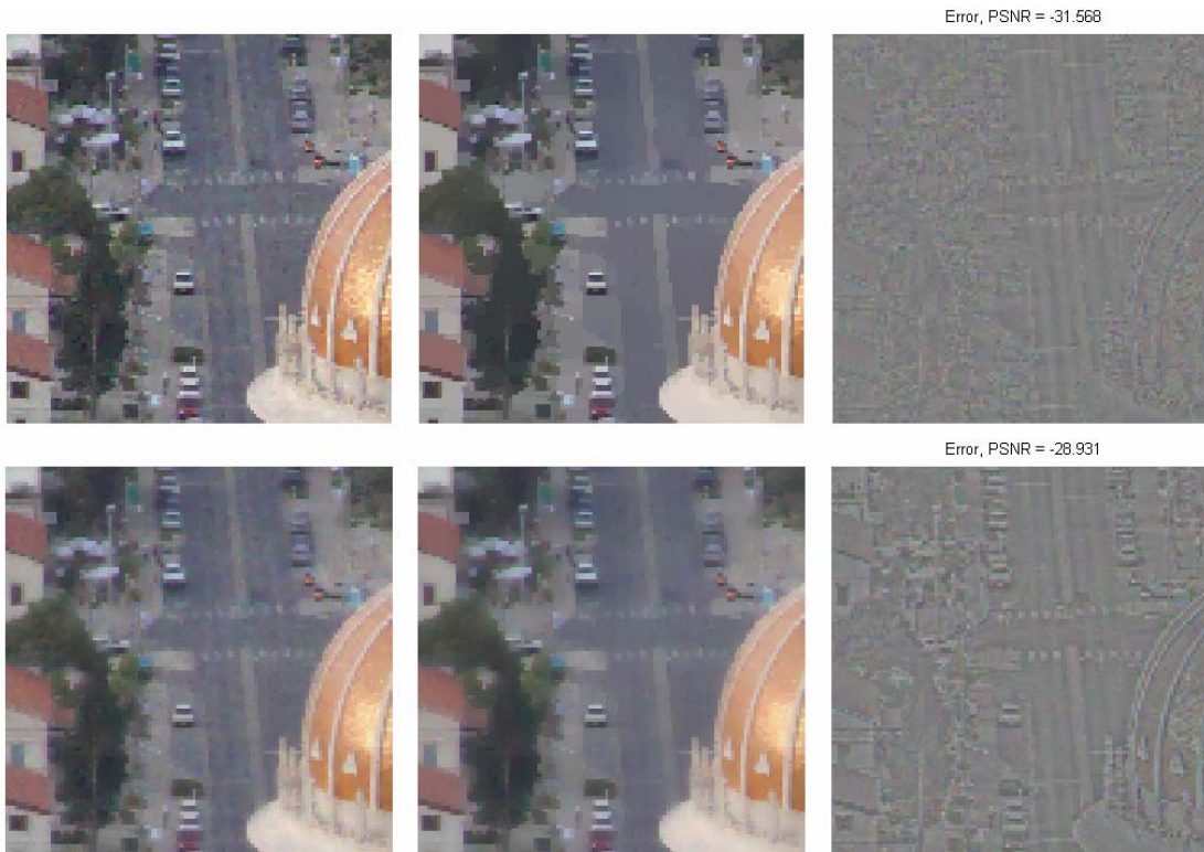
Figure 3: Top row: elastic sheet, 5D color representation. Bottom row: complex diffusion. From left to right: result image after 50 iterations, result image after 100 iterations, error image after 100 iterations.
