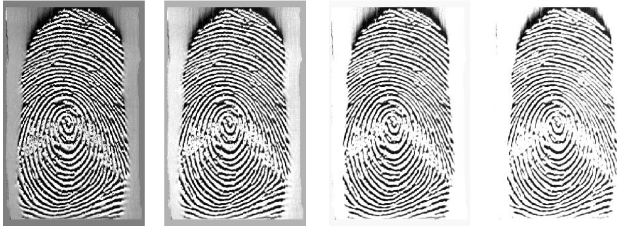
Fig. 3. Example of anisotropic smoothing of a low-quality fingerprint image. From left to right: noisy original, and images after 1, 2 and 3 iterations.
