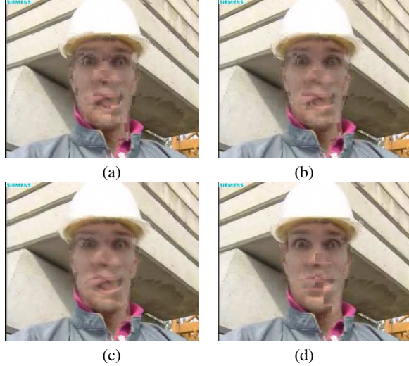
Fig. 3. The interpolated results of frame 94 of FOREMAN sequence. (a), (b), (c), and (d) are the results produced by Direct MCFI, vector median filter in [1], MV smoothing in [2], and MV selection described in [3] respectively
