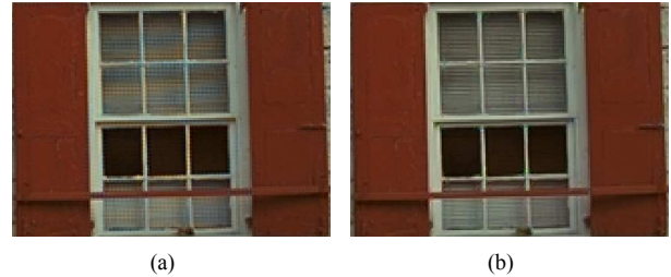
Fig. 5. Reconstruction from the Bayer mosaic (left) and from a pseudo-random mosaic (right), illustrating the false color suppression of the pseudo-random mosaic.
