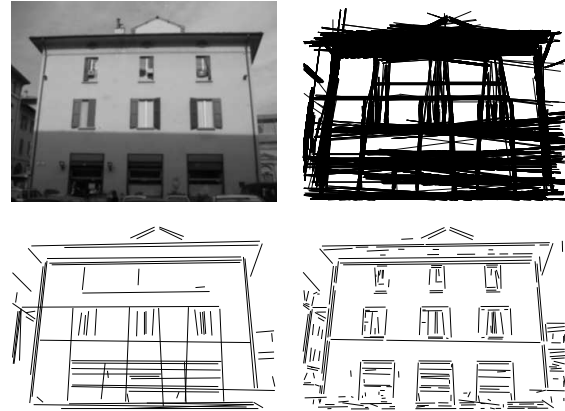
Fig. 1. Up-Left: A digital image. Up-Right: All DMM 1-meaningful segments. Clearly there are many more printed segments than we can perceive, but all of them we do perceive are among these detected segments. Bottom-Left: DMM 1-meaningful segments after exclusion principle. Bottom-Right: Multisegment detections (the proposed method).
