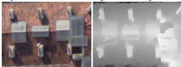
Fig. 1. Image and DEM crops featuring chimneys and glass roofs.
