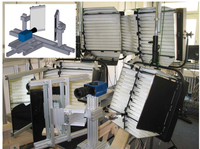
Fig. 1. High speed camera and mirror construction with two surface mirrors. Top Left Corner: Schematic scheme of the construction.
