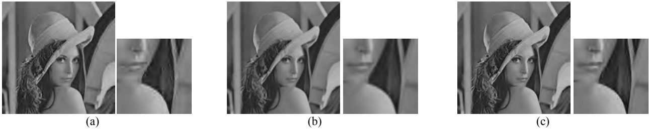
Figure 7 Lena at 0.1 bpp. (a) JPEG2000 (PSNR: 30.46dB). (b) Bicubic Up-sampling (PSNR: 28.75dB) (c) Our scheme (PSNR: 31.25dB).
